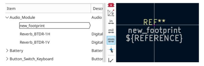
These items are centered on the footprint's anchor (origin point), which is indicated with a magenta cross symbol. The anchor can be repositioned (changing the (0, 0) point for the footprint) by selecting the 400 button and clicking on the new desired anchor position.
