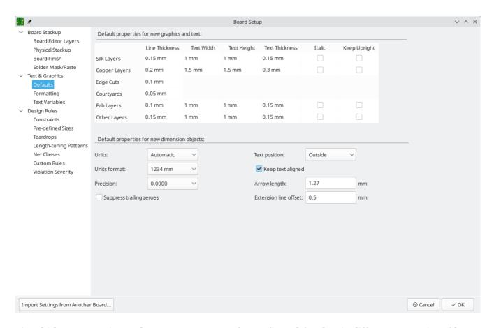
Line thickness, text size, and text appearance can be configured for the six different categories of layers shown in the dialog. Additionally, the properties for dimension objects can be configured for all layers. For more details about dimension properties, see the Dimensions section below.
