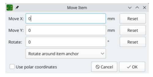
To position a footprint relative to another object, you can use the Position Relative tool (Shift + P). With this tool, you select a reference point for the move, which can be the local origin, the grid origin, or another arbitrary point, such as a pad in another footprint. The selected footprint is moved to the specified offset from the reference point.
