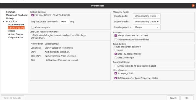
Flip board items L/R: Controls the direction board items will be flipped when moving them between the top and bottom layers. When checked, items are flipped Left-to-Right (about the Vertical axis); when unchecked, items are flipped Top-to-Bottom (about the Horizontal axis).
