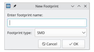
The name will set the name of the footprint, which is used when assigning a footprint to a symbol, and is also used as the filename of the footprint file on disk.
