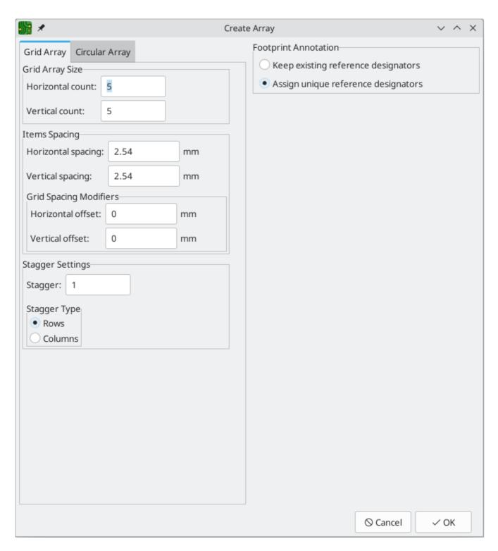
**Grid Arrays** are rectangular and are described by a **horizontal count** and a **vertical count**, which set the number of columns and rows in the array, respectively. The **horizontal** and **vertical spacing** settings describe the distance between columns and rows, while the **horizontal** and **vertical offset** settings describe a shift applied to each row/column compared to the previous row/column.
