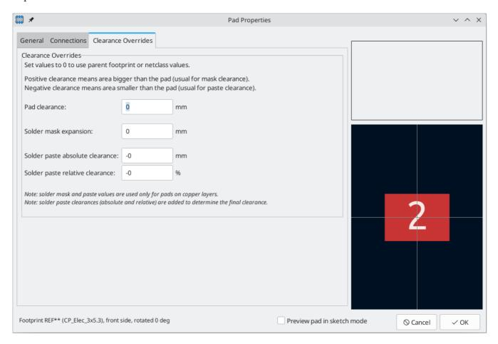
**Pad clearance** controls the minimum clearance between the pad and any copper shape (tracks, vias, pads, zones) on a different net. This value is normally set to 0 which will cause the pad clearance to be inherited from any clearance override set on the footprint, or the board's design rules and netclass rules if the footprint clearance is also set to 0.
