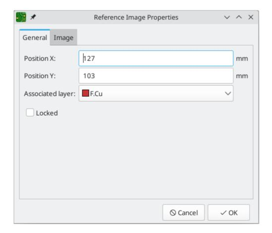
Reference images have an associated layer; they are shown and hidden along with this layer. The layer initially associated with a reference image is the layer that was active when the image was added. You can change the associated layer in the image's properties.
